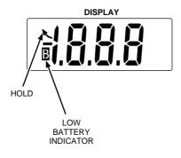
To ensure proper operation of the meter, immediately replace the battery when the low battery indicator appears.
